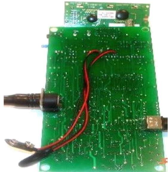
Fig. 22. Development board—Solder side.
