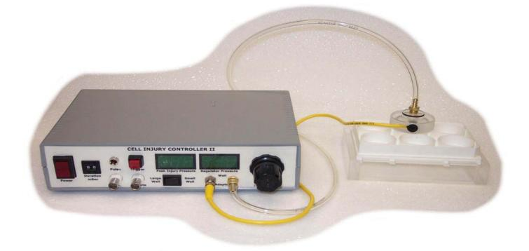
The **Cell Injury Controller II** (CIC II) is an electronically controlled pneumatic device providing all the control and measurement functions necessary to for producing strain induced trauma to *in vitro* cell cultures. The CIC II facilitates study of morphologic, physiologic and biochemical responses of cultured cells to strain induced trauma.
