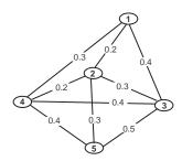
Fig. 1. An example graph modeling a sensor network of five nodes, with the real numbers associated with the edges being the range distances.
