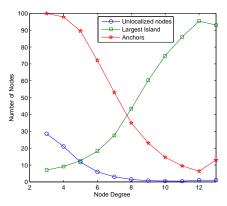
Fig. 9. The numbers of the nodes that are localized in the largest island and that are unlocalized, and the number of anchors required to physically localize the network.
