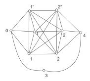
Fig. 3. An example network that requires two rounds of communications in order for the packets to be routed from 0 to 4 via the shortest path.
