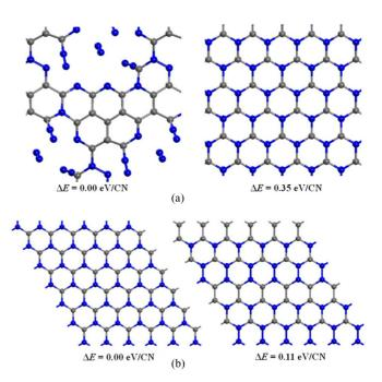
FIG. 1. (Color online) Structure and relative energy of the lowest-energy (left panel) and ordered pattern (right panel) state of h-CN in (a) neutral and (b) hole-doping (p = 0.3) state.
