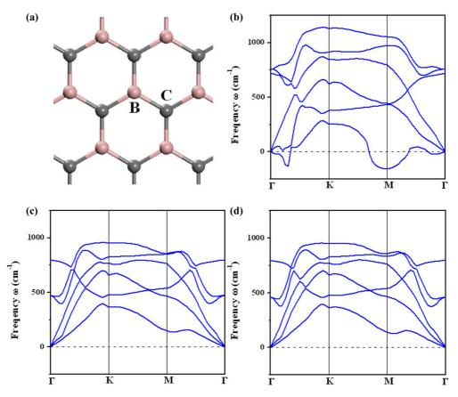
FIG. 6. (Color online) (a) Geometrical structure of the *h*-BC sheet. Phonon dispersion of *h*-BC in (b) neutral and strain-free state, (b) n = -0.2 |e|/unit cell,  $\varepsilon = 5\%$  state, and (c) n = -0.3 |e|/unit cell,  $\varepsilon = 5\%$  state.
