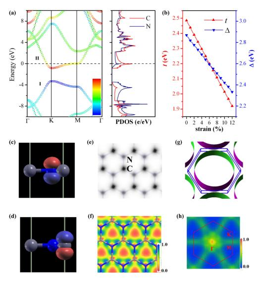
FIG. 4. (Color online) (a) Band structure and PDOS of h-CN sheet with p=0.3 and  $\varepsilon=10\%$ . Blue (red) color represents the state contributed by N (C) atom. (b) Variation of t and  $\Delta$  under different strain. (c, d) MLWFs of band I and II with  $p_z$  characteristics. Slice form of (e) simulated STM image and (f) ELF of the system. (g) Fermi surface pocket and (h) nesting function  $X_q$ .
