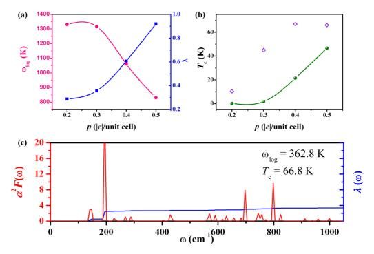
FIG. 5. (Color online) (a) Variation of  $\omega_{\log}$  and  $\lambda(\omega)$  with different doping level under 10% tension. (b) Calculated  $T_c$  with different doping level of h-CN sheet. Solid dot: under 10% tension; empty diamond: under maximum tension. (c) Calculated  $\alpha^2 F(\omega)$  and  $\lambda(\omega)$  of h-CN sheet under p = 0.4 and  $\varepsilon = 15.6\%$ .
