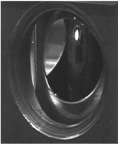
FIG. 5. (Color online) White light emitted for the R-G-B MQD structure represented in Fig. 4. The sample was mounted on the cold finger of a Janis cryostat, which can be clearly distinguished in the figure.
