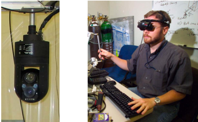
Fig. 4. Camera gimbal and user with visor.
