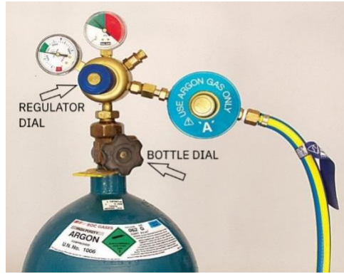
Figure 9: Controlling argon flow
