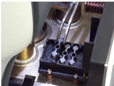
Figure 15: Loading the Simmer Plate
