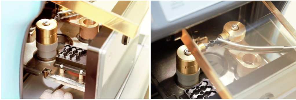
Figure 11 (a, b): Installing the Pulmotec™ (Crucible) into the TP Drawer
