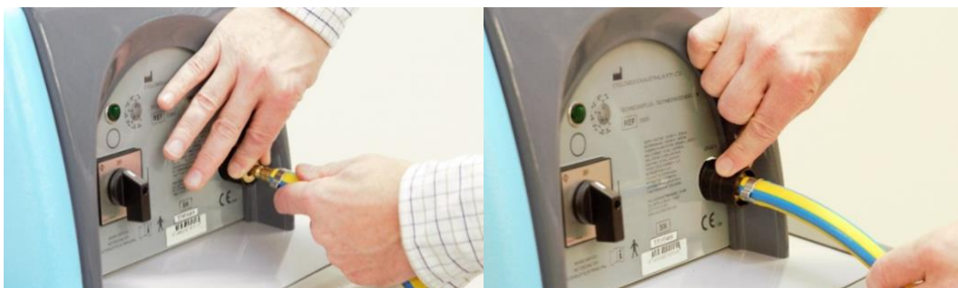
Figure 6(a, b): Connecting the argon supply hose
