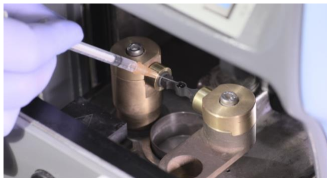
Figure 12: Loading 99m Tc sodium pertechnetate into the Pulmotec™ (Crucible)
