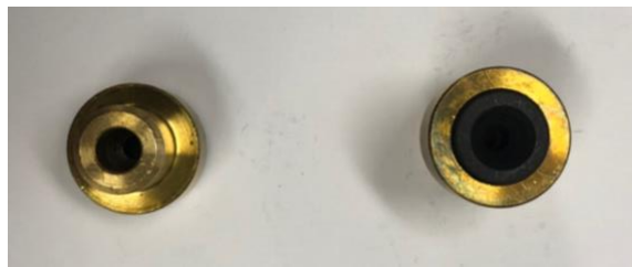
Figure 17: Technegas™ Contacts made from brass with a carbon inlay.
