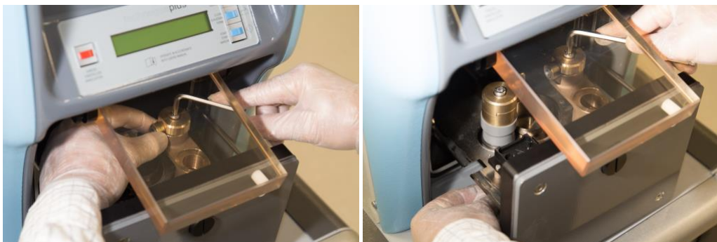
Figure 16: Replacing the Technegas™ Contacts
