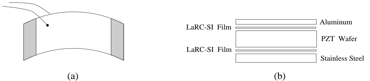
Figure 1. (a) Schematic of a THUNDER actuator; (b) Layers employed in the construction of the composite.
