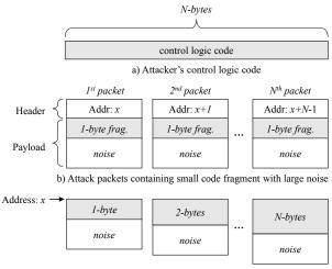
c) PLC protocol address space after all the packets are transferred
