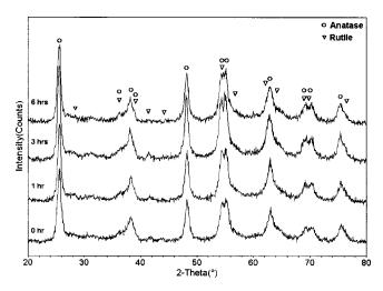
FIG. 1. X-ray diffraction patterns of the as-prepared (0 h) sample of  $\text{Co}_x \text{Ti}_{1-x} \text{O}_{2-\delta}$  and the sample hydrogenated for 1, 3 and 6 h at 573 K. The expected line positions for the anatase and rutile phases are shown.
