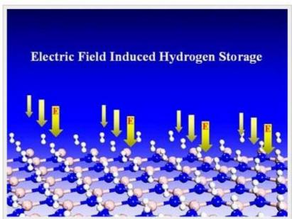
This image illustrates that an applied electric field polarizes hydrogen molecules and the substrate, inducing hydrogen absorption with good thermodynamics and kinetics. Image courtesy of  $\underline{\text{Oian Wang}}$ , Ph.D./VCU.
