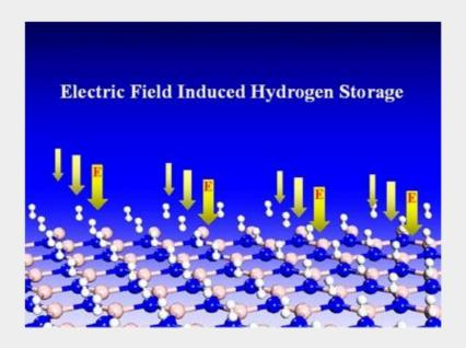
This image illustrates that an applied electric field polarizes hydrogen molecules and the substrate, inducing hydrogen absorption with good thermodynamics and kinetics. Image courtesy of Qian Wang, PhD./VCU.
