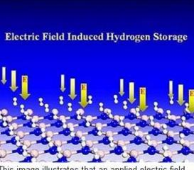
This image illustrates that an applied electric field polarizes hydrogen molecules and the substrate, inducing hydrogen absorption with good thermodynamics and kinetics. Image courtesy of Qian Wang, Ph.D./VCU.
