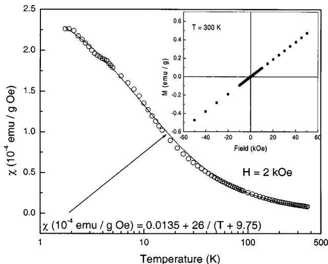
FIG. 2. Temperature dependence of the magnetic susceptibility of the as-prepared sample of  $\text{Co}_x\text{Ti}_{1-x}\text{O}_{2-\delta}$ . The solid line is fit to the equation shown. In the inset is the  $M$  vs  $H$  variation at 300 K.
