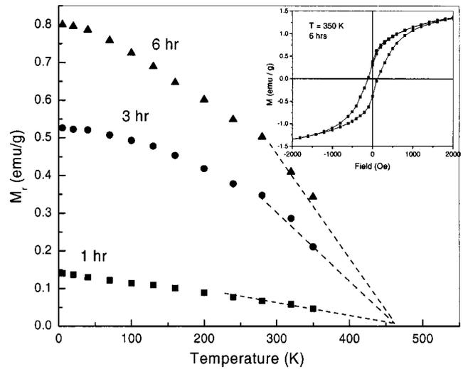
FIG. 3. Temperature variation of remanance  $M_r$  of the sample hydrogenated for 1, 3 and 6 h at 573 K. The dotted lines are extrapolations, indicating  $T_c \approx 470$  K where  $M_r$  goes toward zero. In the inset, the hysteresis loop for the 6 h sample at 350 K is shown.
