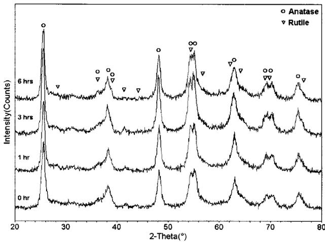
FIG. 1. X-ray diffraction patterns of the as-prepared (0 h) sample of  $\text{Co}_x\text{Ti}_{1-x}\text{O}_{2-\delta}$  and the sample hydrogenated for 1, 3 and 6 h at 573 K. The expected line positions for the anatase and rutile phases are shown.
